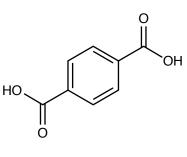
**Explanation:** The structure is terephthalic acid which is mixed with glycol to make PET (polyethylene terephthalate).
