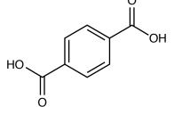
**Explanation:** The structure is terephthalic acid which is mixed with glycol to make PET (polyethylene terephthalate).
