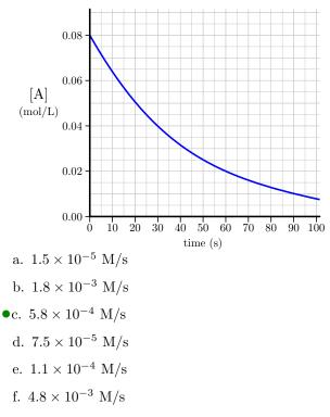
**Explanation:** The absolute value of the tangential slope at 50 seconds is  $5.8 \times 10^{-4}$  M/s. A line from (25s,0.04M) to (85s,0.005M) is a good version of the tangential line to use. This is shown below:
