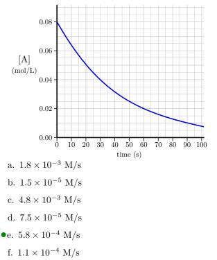
**Explanation:** The absolute value of the tangential slope at 50 seconds is  $5.8 \times 10^{-4}$  M/s. A line from (25s,0.04M) to (85s,0.005M) is a good version of the tangential line to use. This is shown below:
