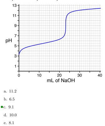
**Explanation:** The endpoint volume is easily seen at 23 mL. The center of the vertical rise is at 9.1 (this is the best number of those listed).
