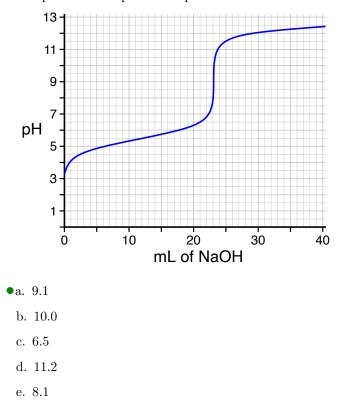
**Explanation:** The endpoint volume is easily seen at 23 mL. The center of the vertical rise is at 9.1 (this is the best number of those listed).
