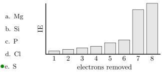
**Explanation:** It is clear that the first 6 electrons follow an increasing trend and then there is a big jump on the 7th. This will only match well with sulfur and it's 6 valence electrons (3s<sup>2</sup>3p<sup>4</sup>). The 7th electron is a 2p electron and is much more difficult to remove to to its closer position to the nucleus.
