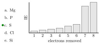
**Explanation:** It is clear that the first 6 electrons follow an increasing trend and then there is a big jump on the 7th. This will only match well with sulfur and it's 6 valence electrons  $(3s^23p^4)$ . The 7th electron is a 2p electron and is much more difficult to remove to to its closer position to the nucleus.
