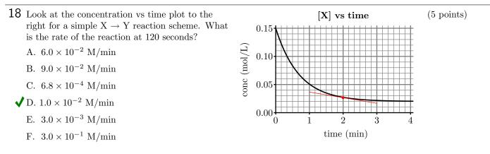
**Explanation:** The absolute value of the tangential slope at 2 minutes is  $1.0 \times 10^{-2}$  M/min. Notice the red line shown over the graph.
