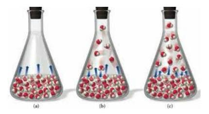
• The Vapor Pressure is a function of the IMF's of the liquid (which results in a higher  $\Delta H_{\text{vap}}$ ) and the temperature.
