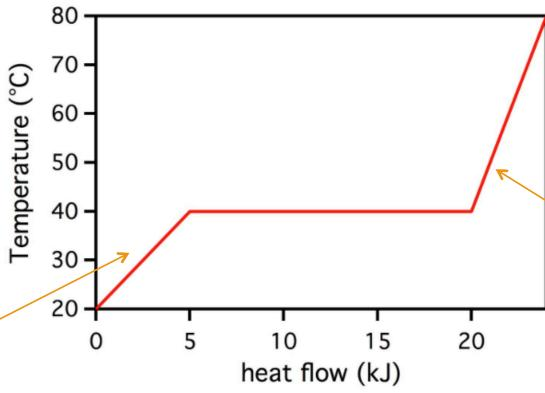
A low heat capacity results in a steeper slope on a heating curve (substance does not do a good job resisting change in temperature when heat is applied)
