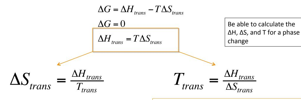
The entropy change of a phase transition given an enthalpy and temperature value
