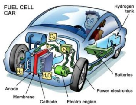
\*  $H_2 + O_2$  gas must be continuously supplied
