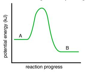
Know HOW to interpret the diagram. How to get  $\Delta E$  and  $E_{\rm a,f}$  and  $E_{\rm a,r}$ . Know transition state theory (activated complex) and how it relates to a potential energy diagram - where does it occur?
