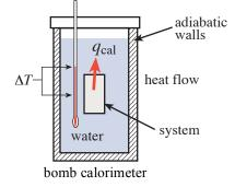
Bomb calorimetry is conducted under constant volume (isochoric) conditions. This is shown explicitly by writing  $q_v$  for the heat term. The subscript "v" means conducted at constant volume. Because the volume is held constant and  $\Delta V$  is forced to be zero, no expansion work can be done throughout the process (w = 0). This means that all heat flow is now equal to the internal
